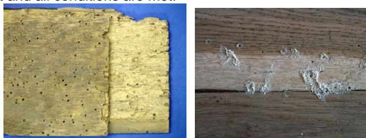
Lyctid powderpost beetle exit holes measure 1/32 – 1/16 inch across.
